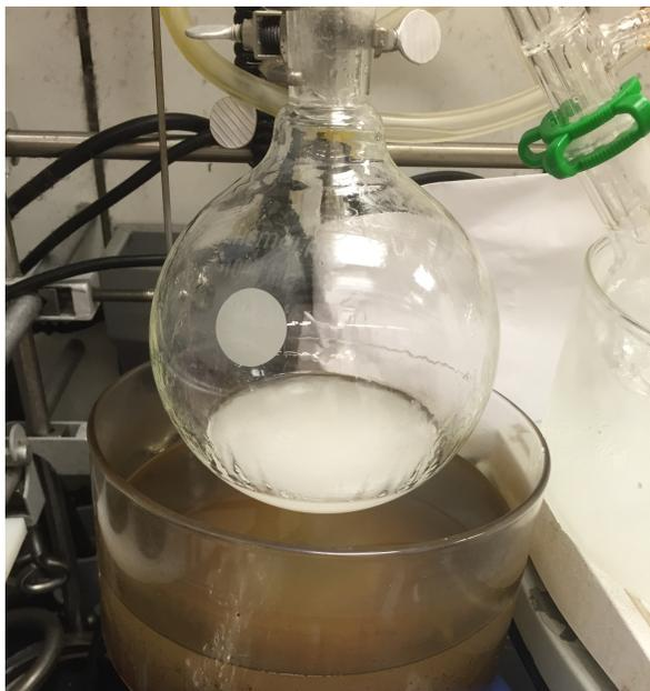
**Figure 4. Semi-Solid Product After Distillation**
